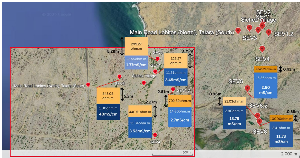
Figure 1: Map of the eight Vertical Electrical Sounding (VES) sites in Sichez. Our analysis led us to recommend site SEV 1.2, near a historic well, as the most promising location for drilling.
