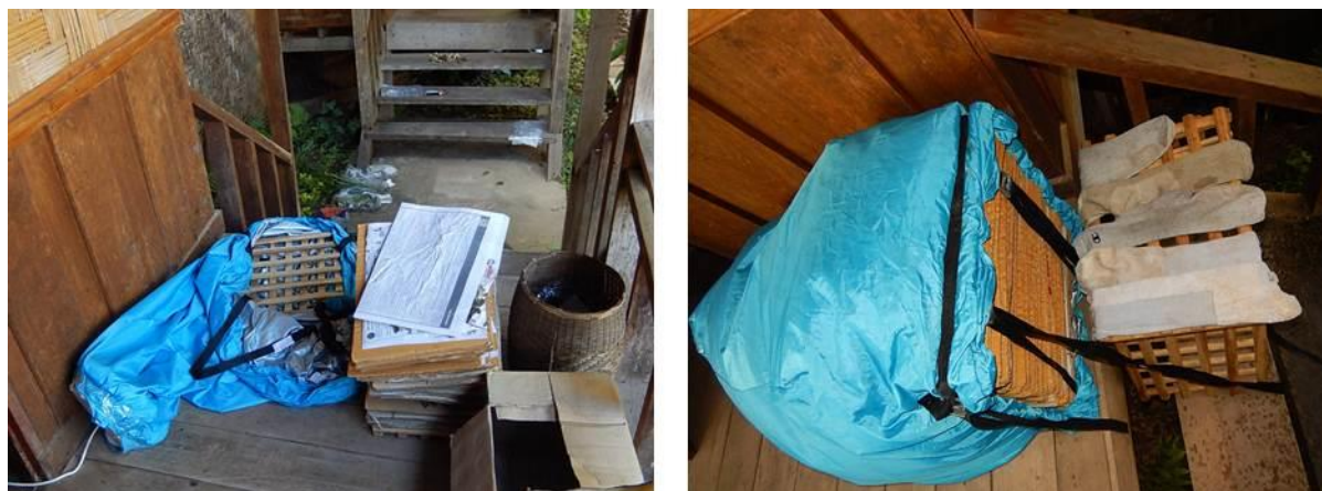
Figure 1. The plant drier used in Lao PDR. An old camping tent was strapped to a small fan heater at one end and to the plant press at the other. Inside the chamber, the silica gel was routinely dried overnight. Left: specimens ready to be pressed and dried. Right: the drier in use (also demonstrating its additional application as socks drier).
