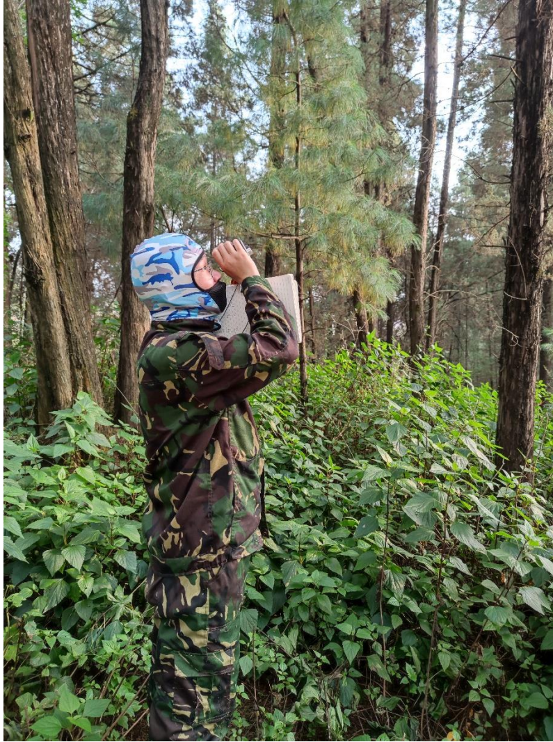
Figure 4. Measuring tree height using Vertex
