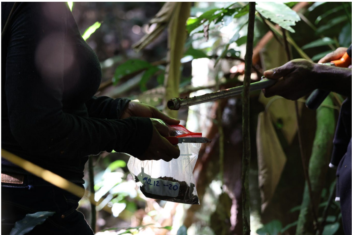
Figure 8. Collection of soil samples. Soils were sampled to 20cm deep using a soil corer. At each location 5 cores were taken and combined.
