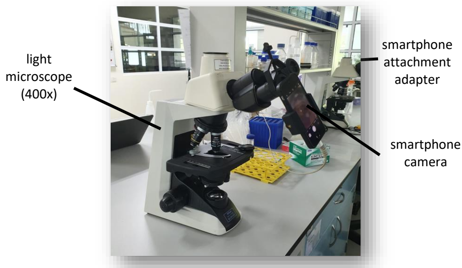
Figure 3. Setup for microscopy and testate amoebae imaging.
