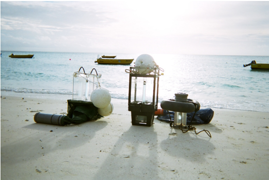
Fig. 3: “Star of Lance”, AIMS and Ecocean light traps ready to be deployed.
