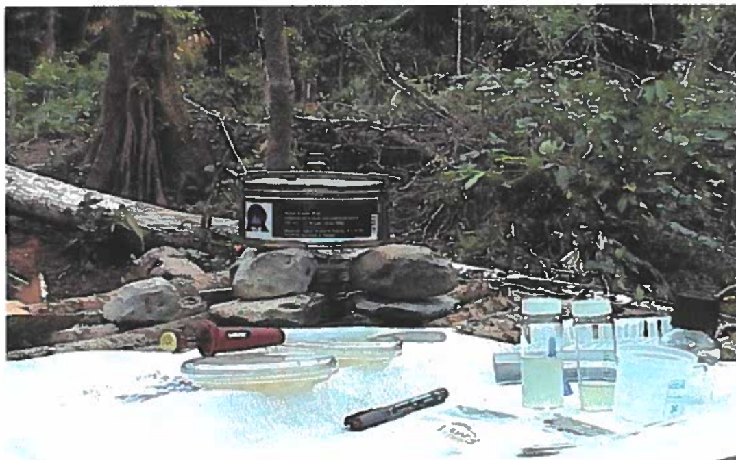
Figure 2. The assay kit including specially designed pressure vessel as well as microbiological media, cultures and other equipment.
