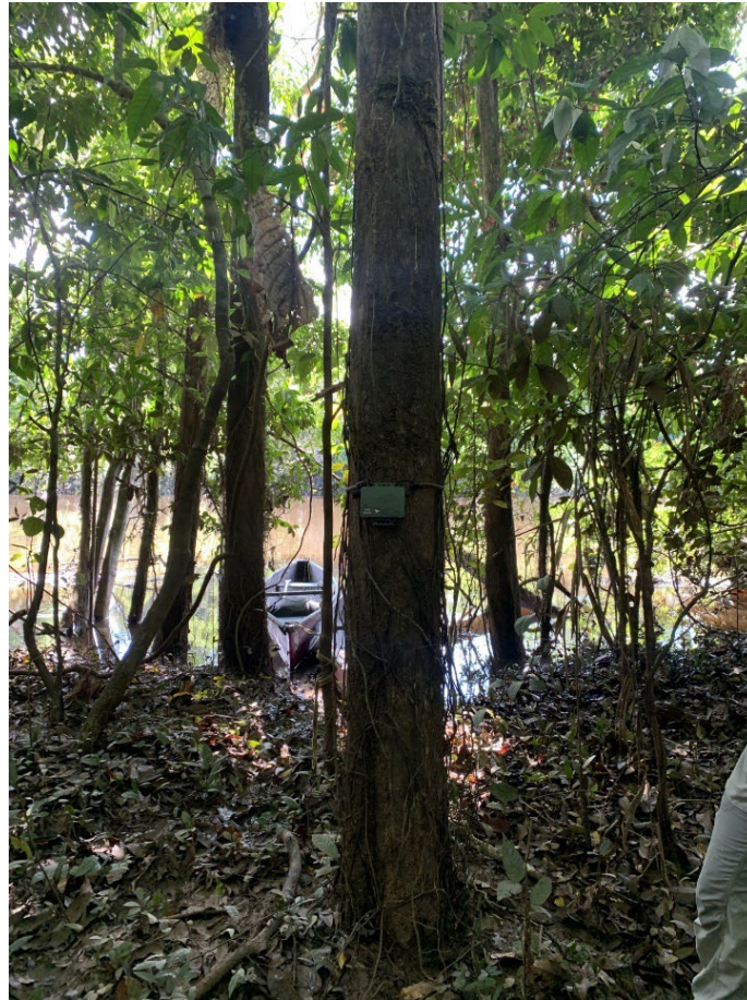
Figure 3. Example monitor placement at chest height, 1-2m above the ground; roughly 3 m in from the bank.
