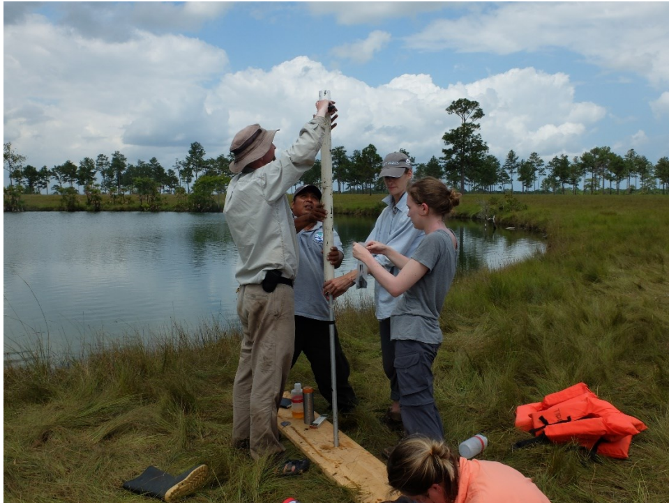
Figure 5: Taking 1cm samples from the mud-water interface core
