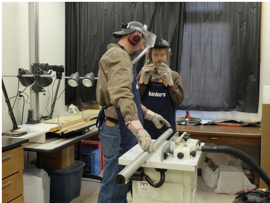
Figure 7 (left): Cutting open the aluminium coring tubes Figure 8 (below left): The sediment inside the core is revealed Figure 9 (below right): Describing the core on a core log
